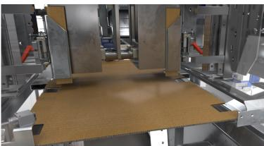
At the active forming section (pictured above), the side panels are fed inward and formed around the mandrel as glue is applied. The body wrap is fed beneath the mandrel, and the sides are folded up and around the side panels as the mandrel deploys downward. Consistent compression is applied to ensure case squareness and a secure glue seal.
