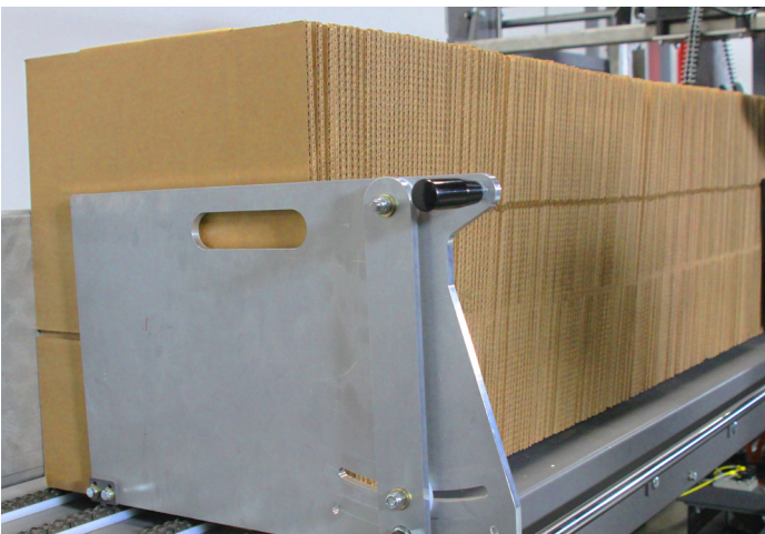
Powered follower maintains consistent pressure to guide knock down cases smoothly into the Case Erector
