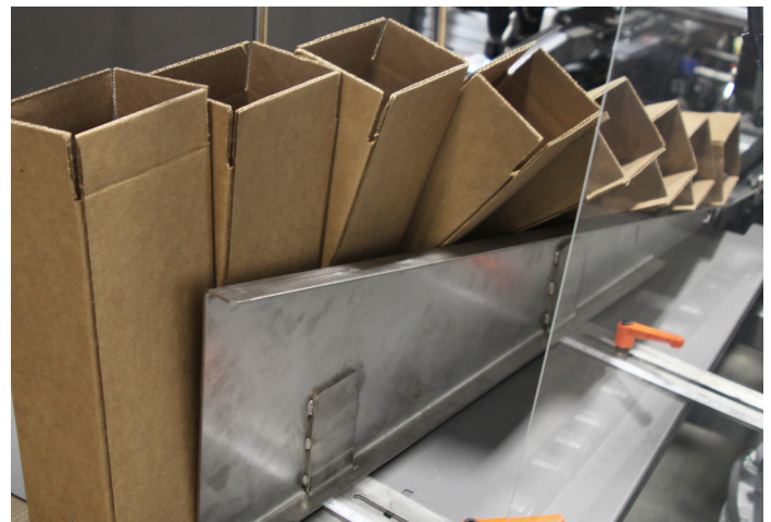
Tall cases move through the outfeed tip up station
